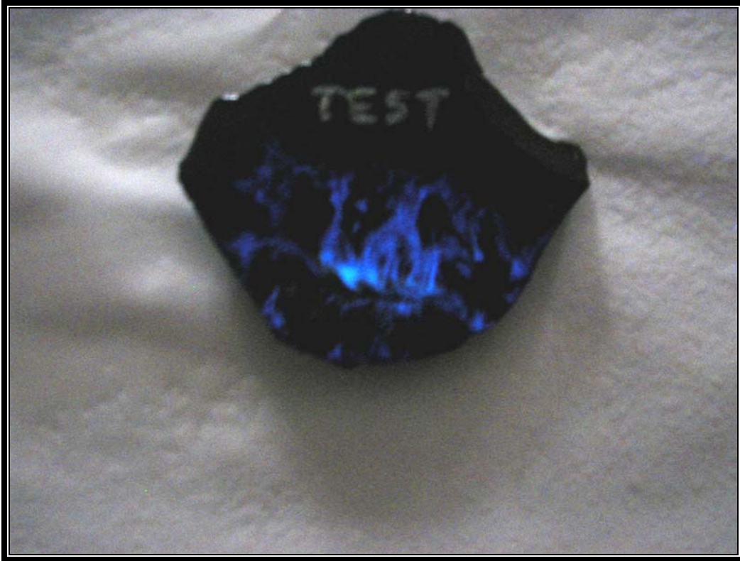
Photograph E-4. Luminescence resultant from positive reaction of reagent with blood.
