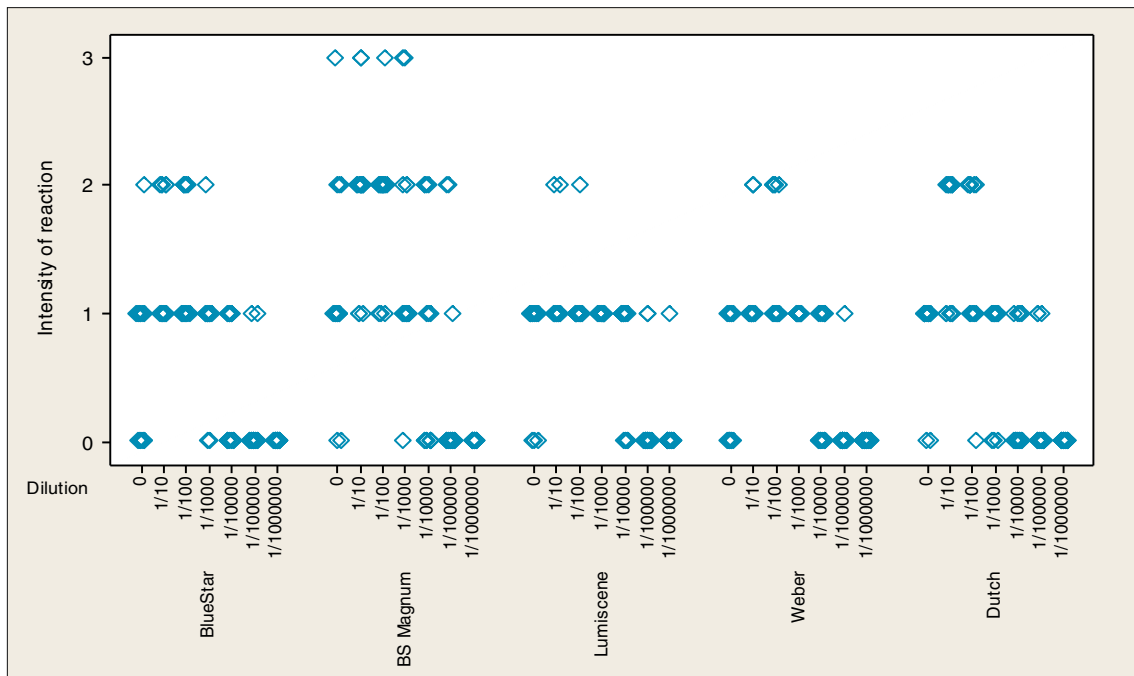
Fig. 1 Comparison of the formulations on fabric at a range of dilutions over 24 h from preparation (x-axis: 0=no reaction; 1=weak/faint; 2=strong/intense; 3=very strong/very intense). Darker data points indicate multiple scores for that variable
