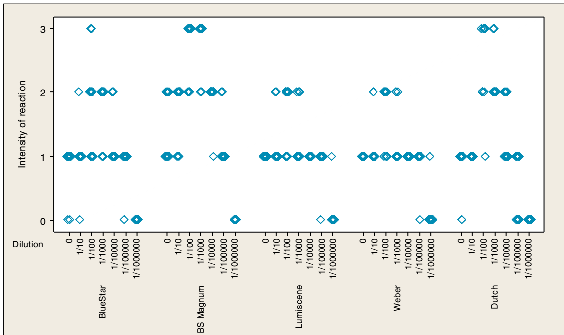
Fig. 2 Comparison of formulations on tile at a range of dilutions over 24 h from preparation (x-axis: 0=no reaction; 1=weak/faint; 2=strong/intense; 3=very strong/very intense). Darker data points indicate multiple scores for that variable
