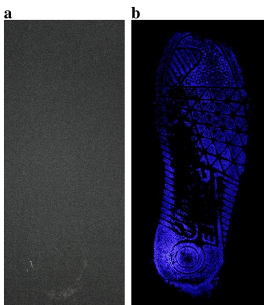
Fig. 14. Enhancement of a footwear impression in blood on black nylon/lycra using luminol: (a) before; (b) after.
