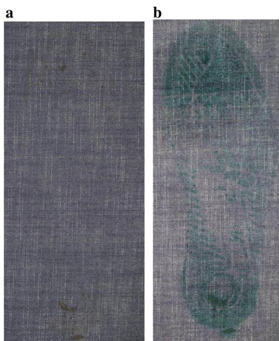
Fig. 9. Enhancement of a footwear impression in blood on denim using LMG: (a) before; (b) after.
