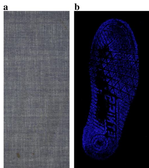
Fig. 13. Enhancement of a footwear impression in blood on denim using luminol: (a) before; (b) after.
